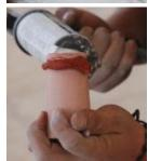
CorPlug has been tested up to 2-hour construction per ESR-3939 when using 3M Fire Barrier Sealant CP 25WB+
